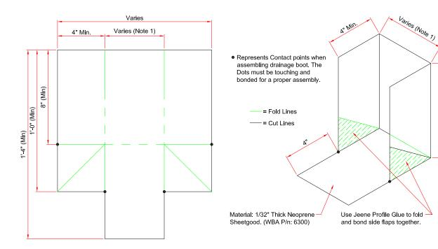
1. Overall width of Boot Transition will be determined on the amount of movement the WSW system can accommodate during normal movement ranges. WBA suggests that the dimension will be at least Maximum Opening plus 1". This is to ensure that there will not be any damage to the boot while the system is at maximum opening.
